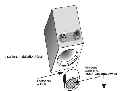
During the Installation and/or Replacement of the MFC, **Membrane** surface **MUST ALLWAYS <u>FACE</u>** *DOWNWARD*, and the Contact side of the Membrane, **MUST** be placed **FIRST** into Analysis Unit.
